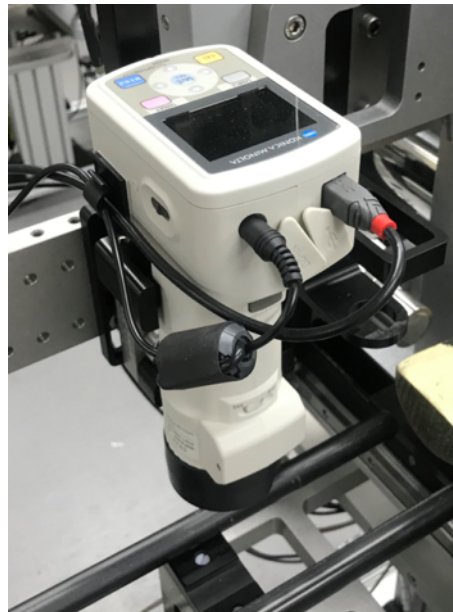
Figure 1: Konica Minolta visible light spectrophotometer
