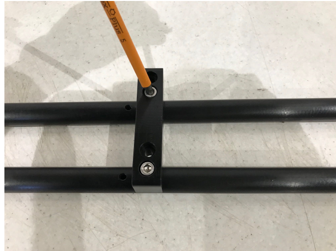
Figure 3.3: Switch over the rails to the narrow gauge sleeper threads. Remove only one rail at a time.
