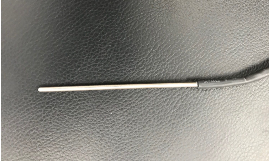
Figure 1: Platinum Resistance Thermometer used on the MSCL-S System
