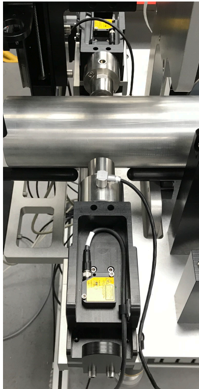
Figure 1: Core thickness laser measurement system
