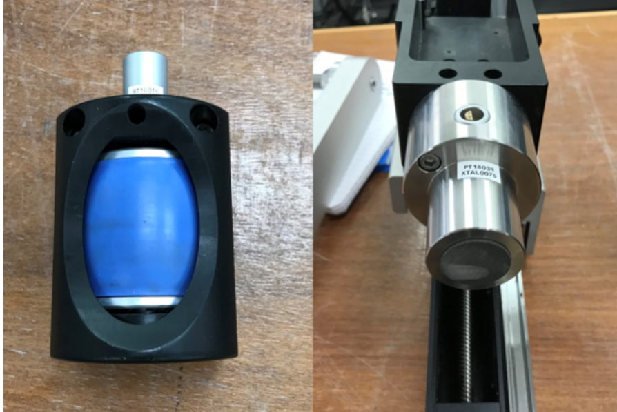
Figure 1: ARC rolling transducer (left), piston transducer (right)
