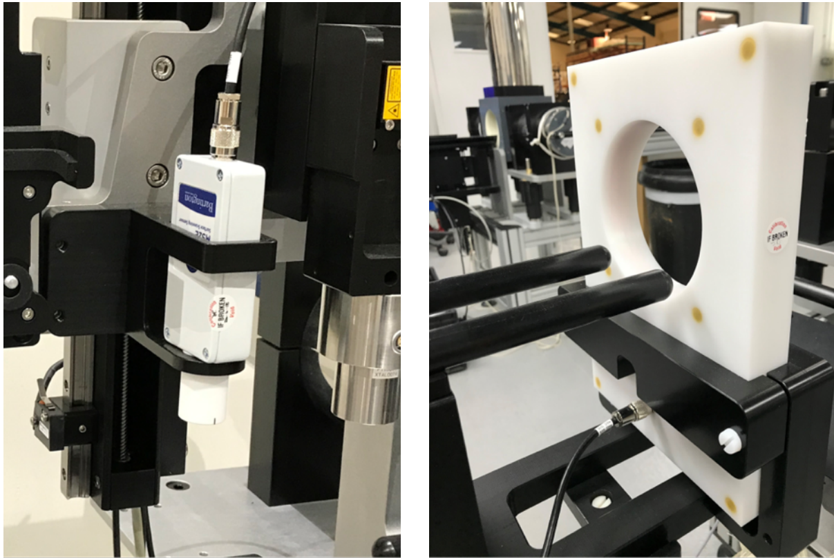
Figure 1: Bartington point (left) and Bartington loop (right) magnetic susceptibility sensors
